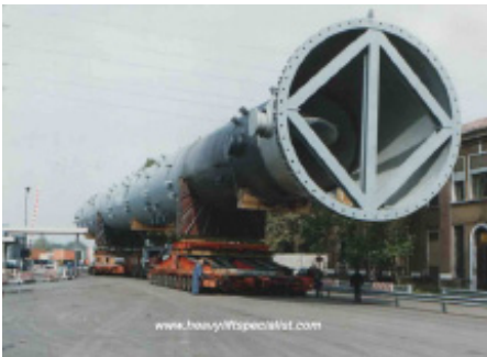
Transport & shipment of a 93 m long and 725 ton heavy CO2 splitter from Pt. Marghera, Italy to the Quatum Refinery in Houston, USA.
